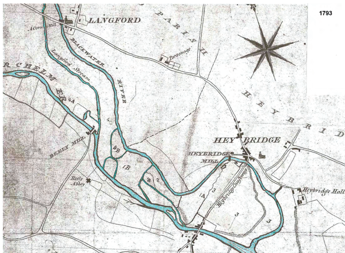
FIGURE 1: Based on ERO Q/RUM 1/4 this version of the map has had the proposed canal removed. The final route of the canal made use of the course of the Blackwater river and not between the two rivers as first proposed. Reproduced by courtesy of the Essex Record Office.
