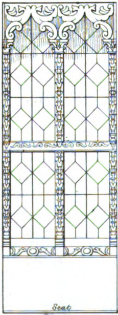
Interior Elevation of Window. (in Terra Cotta)
