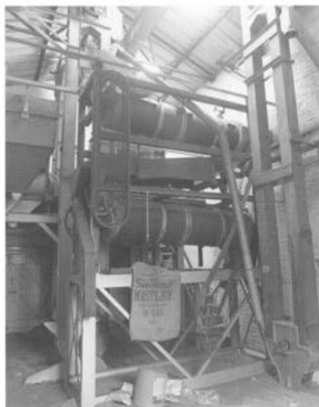
Plate 10 Malthouse No. 4, Boby seed screening machines.
