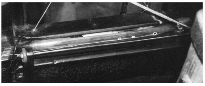
Plate 2. A fly-shuttle gear fitted to a loom at Quarry Bank Mill in Styal, Cheshire. (Author's photograph by permission of the National Trust).
