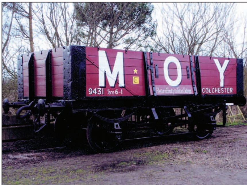
7. A 'Moy Colchester' railway wagon located at Brockford Station, Wetheringsett, Suffolk. This wagon is a 5-plank coal wagon no. 9431. The words on the side 'return empty to Toton sidings' means it was sent to Toton marshalling yards to be loaded with coal. Although not authentic for this type of wagon, it was fitted with automatic brakes so it could be run in passenger trains. (Photograph reproduced by courtesy of the Mid-Suffolk Light Railway Museum)
