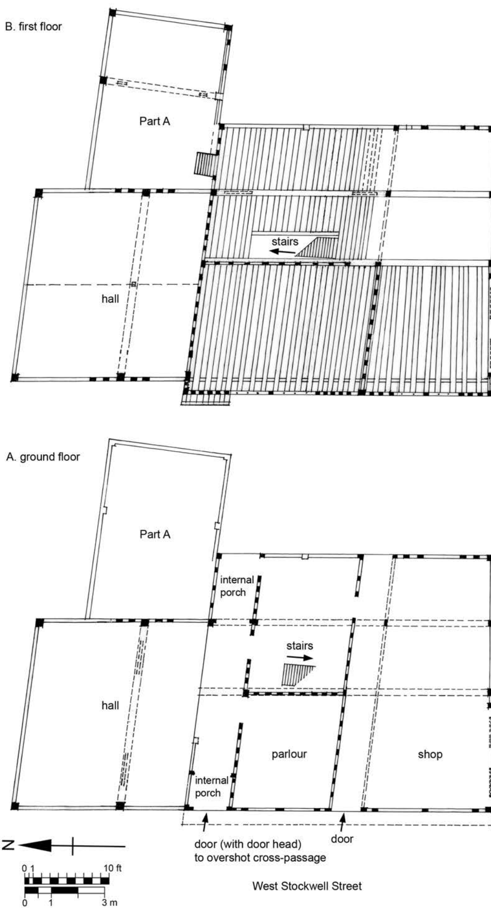
FIGURE 369: Schematic plan showing the components of 3–6 West Stockwell Street (corpus no. 98), (bottom) a. ground floor, (top) b. first floor
