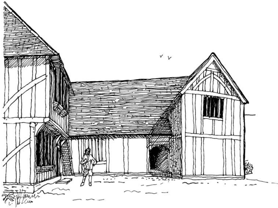
FIGURE 350: Isometric reconstruction of 7–9 Trinity Street (corpus no. 93), Tymperleys, from the rear (west), showing (from the left) parlour / solar (C / D), hall (A) and service wing (B) (not to scale)
