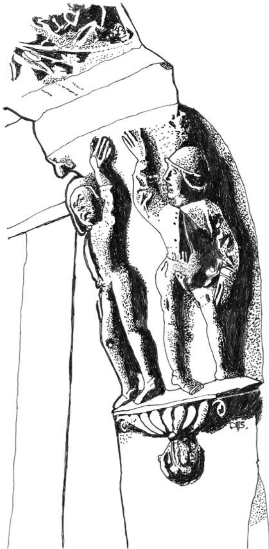
FIGURE 255: Finely carved brackets supporting the bridging joist in the rear wing of The Marquis of Granby, 24 North Hill (corpus no. 66) (not to scale)
